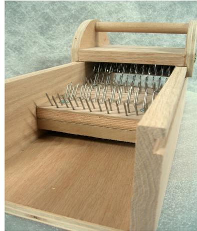
The Fancy Kitty Mini Picker is shipped completely assembled. To use the picker, simply remove the two picker sled stop screws located in the left sled slide (as you are looking at the picker from the feed tray end).
