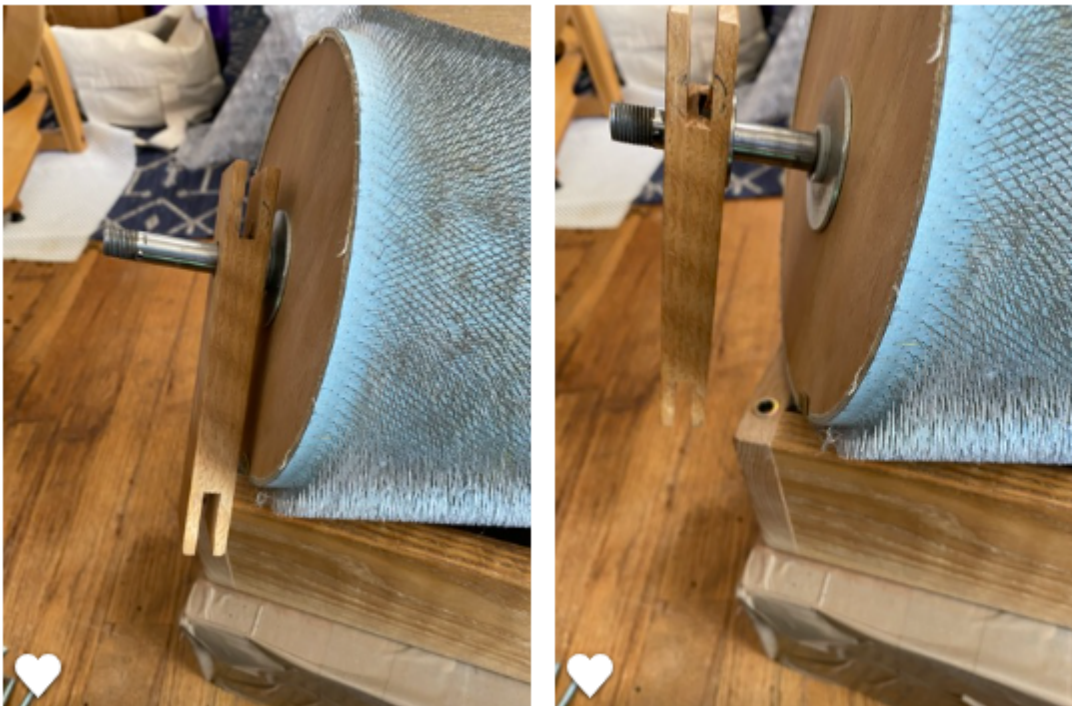
On the handle side, you can slide the grooved brace away from the swift and clean off the axle. (Note: I will never set the swift in this position on the base again—it's potentially risky for the carding cloth teeth.)
