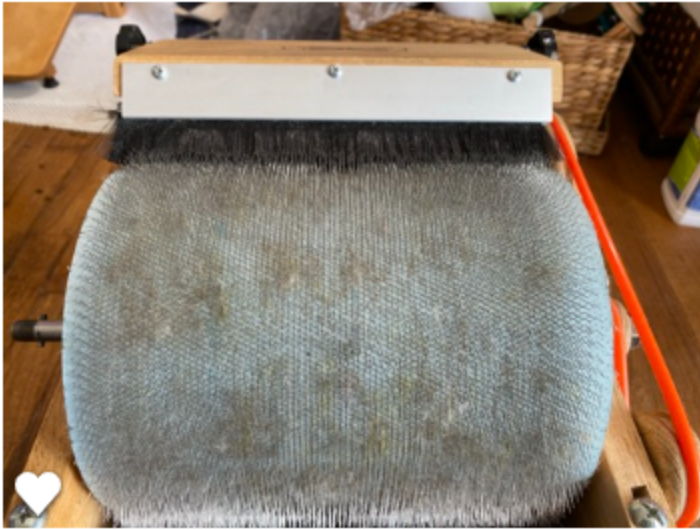
The brush attachment and drive band reinstalled.
